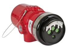
The X3302 with pulse/relay output is designed for use in controller based systems. In addition to use in new systems, it can serve as a direct field replacement for Detector Electronics Corporation's (Det-Tronics) controller based flame detectors that generate a pulse output (not compatible with R7484 and R7409B/C).
